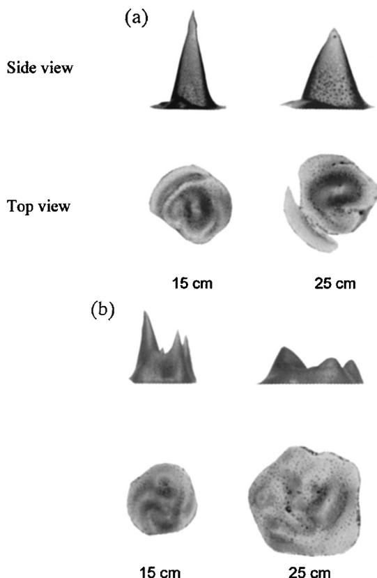
Fig. 14. Output-beam profiles on the 1500-W laser of a 700- $\mu\text{m}$ -bore, 1.54-m-long hollow-glass waveguide (a) straight and (b) bent 360°.
