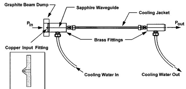
Fig. 4. Structure of hollow-waveguide cooling jacket and Cu input fitting.
