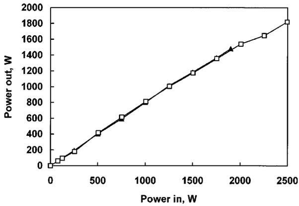
Fig. 8. Transmission of a straight, 1070- $\mu\text{m}$ -bore, 1.2-m-long hollow-sapphire waveguide on the 2000-W laser ( $\blacktriangle$ ) and the 3000-W laser ( $\square$ ).
