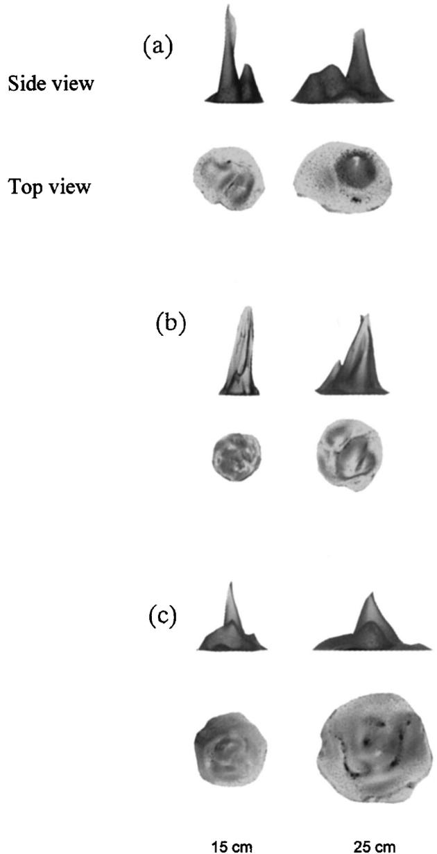
Fig. 10. Output-beam profiles on the 1500-W laser of (a) 790- $\mu\text{m}$ -bore hollow-sapphire and (b) 1070- $\mu\text{m}$ -bore hollow-sapphire waveguides and on the 2000-W laser of (c) 1070- $\mu\text{m}$ -bore hollow-sapphire waveguide.
