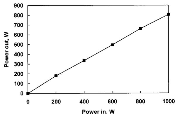
Fig. 7. Transmission of a straight, 1070- $\mu\text{m}$ -bore, 1.5-m-long hollow-sapphire waveguide on the 1500-W laser.
