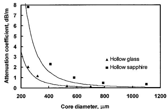
Fig. 1. Theoretical (solid curves) and measured attenuation in straight hollow-glass and hollow-sapphire waveguides at 10.6  $\mu$ m.
