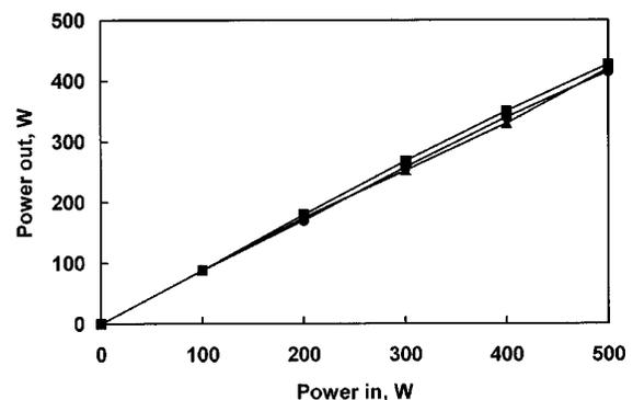
Fig. 13. Transmission of straight (■), bent 90° (▲), and bent 180° (●) 700- $\mu\text{m}$ -bore, 1.54-m-long hollow-glass waveguides.
