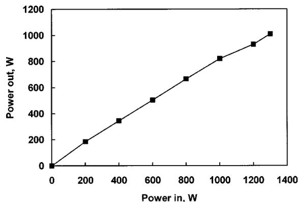
Fig. 11. Transmission of a straight, 700- $\mu\text{m}$ -bore, 1.54-m-long hollow-glass waveguide on the 1500-W laser. The maximum output power was 1010 W.
