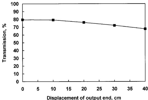
Fig. 9. Bending loss of a 1070- $\mu\text{m}$ -bore, 1.2-m-long hollow-sapphire waveguide a 3000-W laser operating at 500 W.
