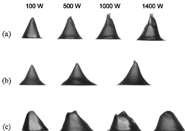
Fig. 5. Beam patterns of (a) 1500-W laser, (b) 2000-W laser, and (c) 3000-W laser taken from burns made in acrylic blocks.
