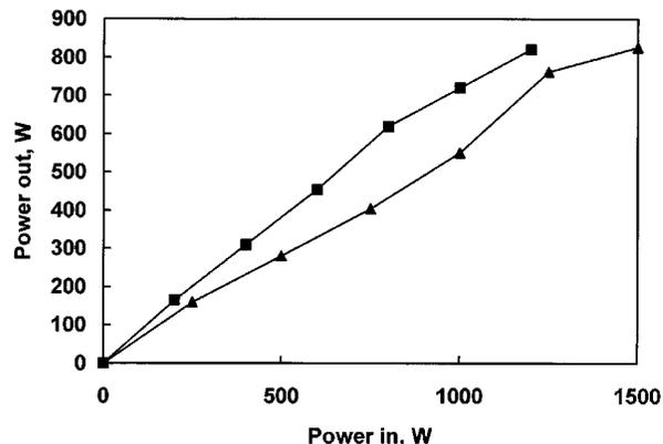
Fig. 6. Transmission of a straight, 790- $\mu\text{m}$ -bore, 1.2-m-long hollow-sapphire waveguide on the 1500-W laser (■) and the 2000-W laser (▲).
