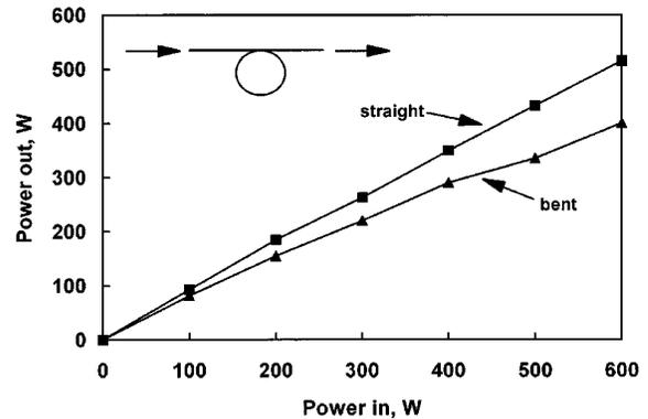
Fig. 12. Transmission of straight (■) and bent 360° (▲) 700- $\mu\text{m}$ -bore, 1.54-m-long hollow-glass waveguides on the 1500 W laser.
