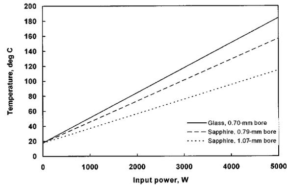
Fig. 3. Calculated temperature of the inner wall at the input end of a 700- $\mu\text{m}$ -bore hollow-glass waveguide (solid line), a 790- $\mu\text{m}$ -bore hollow-sapphire waveguide (dashed line), and a 1070- $\mu\text{m}$ -bore hollow-sapphire waveguide (dotted line) for an attenuation of 3 dB/m. Calculations were based on forced convective water cooling with a water temperature of  $18^\circ \text{C}$ .
