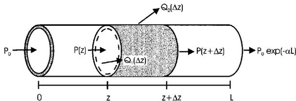
Fig. 2. Diagram showing power lost,  $P(z) - P(z + \Delta z)$ , and heat flow from the outer surface,  $Q_2(\Delta z)$ , and inner surface,  $Q_1(\Delta z)$ , in a waveguide section of length  $\Delta z$ .
