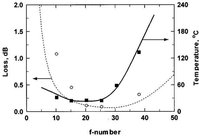
**Fig. 7** Calculated (solid curve) and measured (solid squares) input-end temperature as well as calculated (dashed curve) and measured (open circles) total loss of a 1-m-long, 700- $\mu$ m-bore hollow-glass waveguide under different launch conditions.
