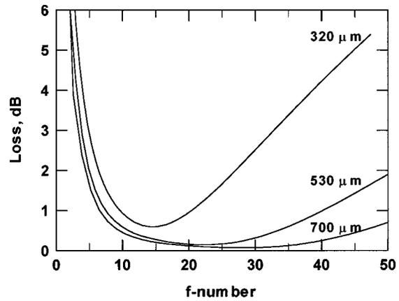
Fig. 5 Minimum-loss coupling conditions for the 1-m-long, 320-, 530-, and 700- $\mu\text{m}$ -bore hollow-glass waveguides.
