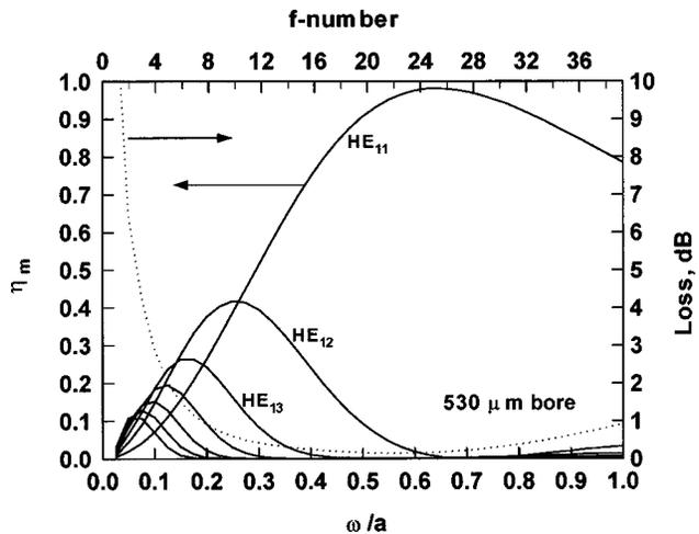
Fig. 3 Calculated coupling coefficients (solid curves) and total loss (dotted curve) of a 1-m-long, 530- $\mu$ m-bore, hollow-glass waveguide.
