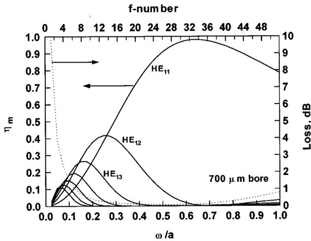
Fig. 4 Calculated coupling coefficients (solid curves) and total loss (dotted curve) of a 1-m-long, 700- $\mu\text{m}$ -bore, hollow-glass waveguide.
