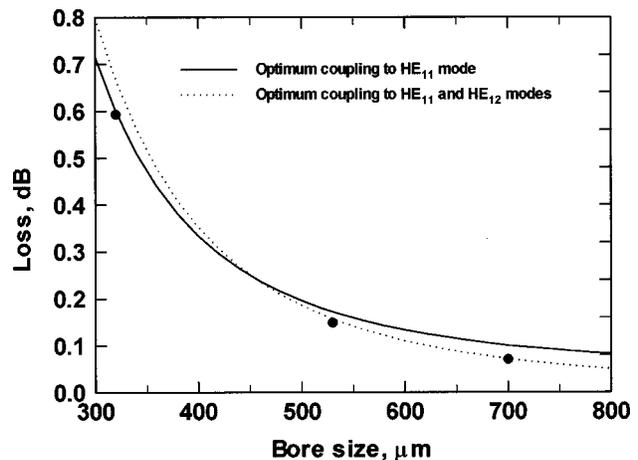
Fig. 6 Total loss as a function of bore size under the launch condition that maximizes the amount of energy coupled to just the  $\text{HE}_{11}$  mode (solid curve) and that maximizes the amount of energy coupled to both the  $\text{HE}_{11}$  and  $\text{HE}_{12}$  modes (dotted curve). The solid circles represent the calculated minimum loss for the three different bore size waveguides.
