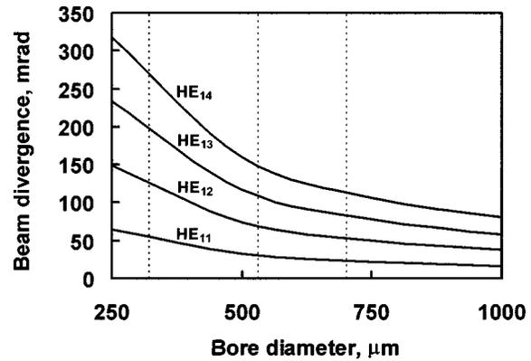
**Fig. 8** Calculated beam divergence of the first four HE<sub>1m</sub> modes exiting a hollow-glass waveguide. The vertical dashed lines indicate the 320-, 530-, and 700- $\mu$ m-bore waveguides.
