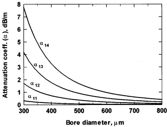
Fig. 1 Calculated attenuation coefficients of the first four HE<sub>1m</sub> modes in hollow-glass waveguides.
