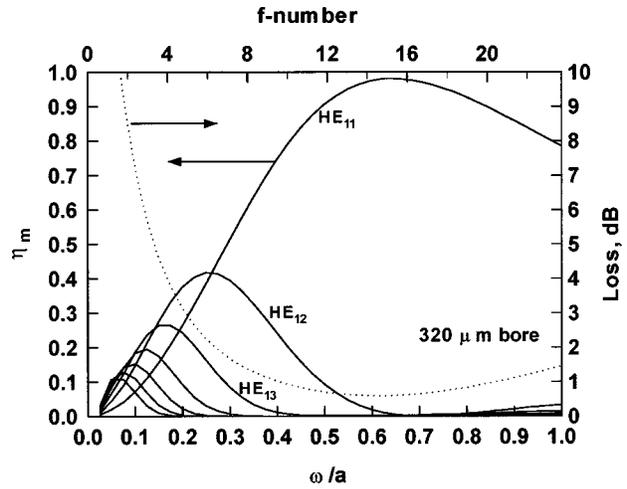
Fig. 2 Calculated coupling coefficients (solid curves) and total loss (dotted curve) of a 1-m-long, 320- $\mu$ m-bore, hollow-glass waveguide.
