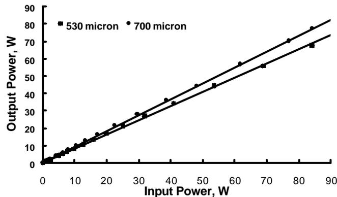
Figure 15 - Low CO<sub>2</sub> laser power delivery for two bore size HGWs with no cooling. This is the typical laser power used in medical lasers and for low power cutting and marking.
