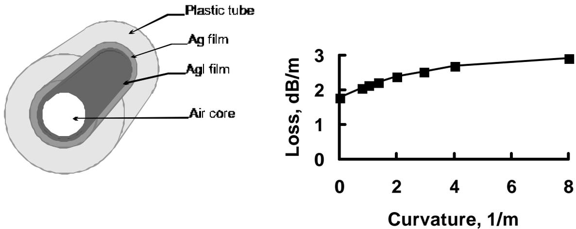
Figure 6 - Structure and bending loss for hollow plastic waveguide made by Croitoru's group at Tel Aviv University. (18)
