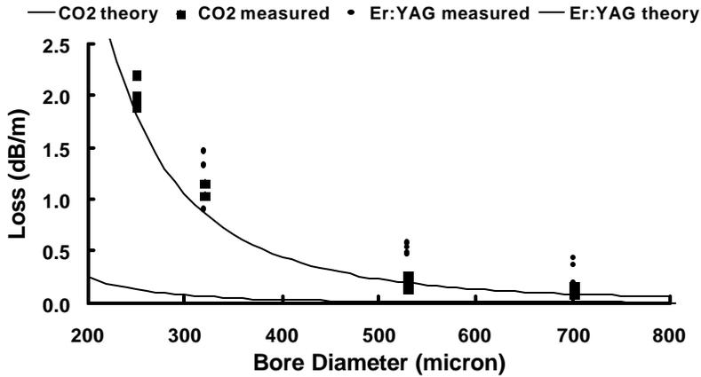
Figure 11 - Measured losses for straight HGWs using CO<sub>2</sub> and Er:YAG lasers. Note that the predicted losses are well below the measured ones at 2.94 μm.
