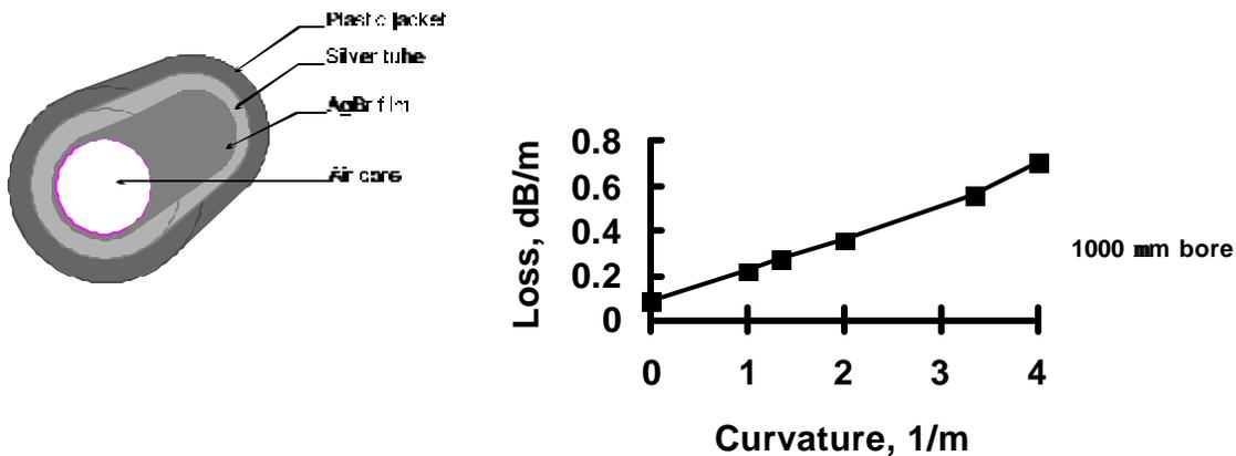
Figure 4 - Structure and bending loss for hollow guide made from silver tubing with a AgBr film deposited on the inside surface. (24)
