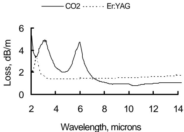
Figure 10- Spectral response of two HGWs; one designed for low loss at the CO<sub>2</sub> wavelength of 10.6 μm and the other for low loss at the Er:YAG laser wavelength of 2.94 μm.
