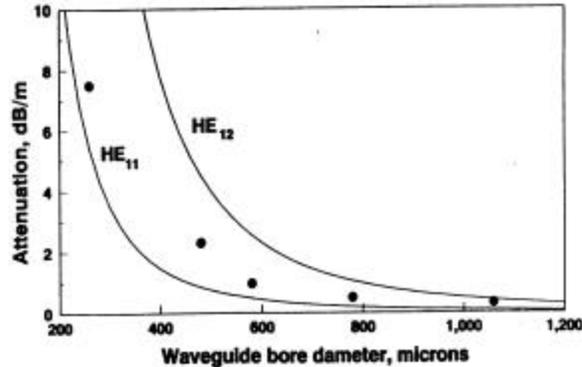
Figure 13 - Measured loss at  $10.6 \mu\text{m}$  for straight, hollow sapphire waveguides. Note that the losses fall between the theoretical losses for the  $\text{HE}_{11}$  and  $\text{HE}_{12}$  modes. This is a result of surface roughness of the sapphire tubing.
