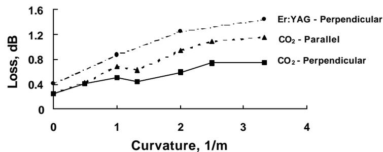
Figure 3 - Losses for bent hollow metallic guides shown in Figure 3 taken at both CO<sub>2</sub> and Er:YAG laser wavelengths. (22)
