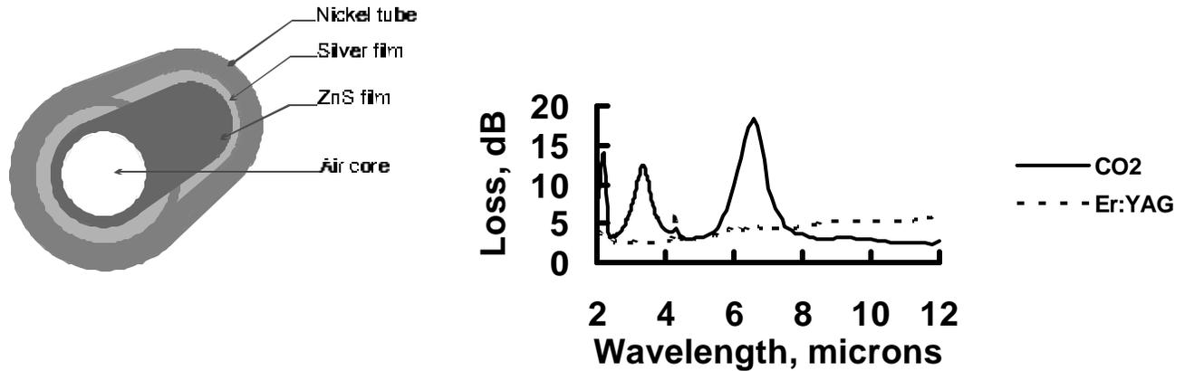
Figure 2 - Structure and spectral losses for metallic waveguide fabricated by Miyagi's group at Tohoku University. (22)
