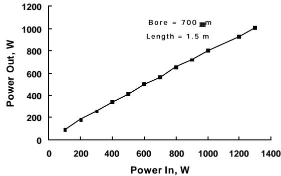
Figure 16 - High CO<sub>2</sub> laser power delivery for a 700 μm bore HGW with a water cooling jacket. Note that the maximum power is just over 1,000 W!
