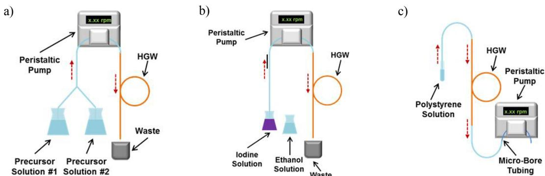
Figure 2 – a) Ag and metal sulfide thin films, b) AgI thin films, c) PS thin films
