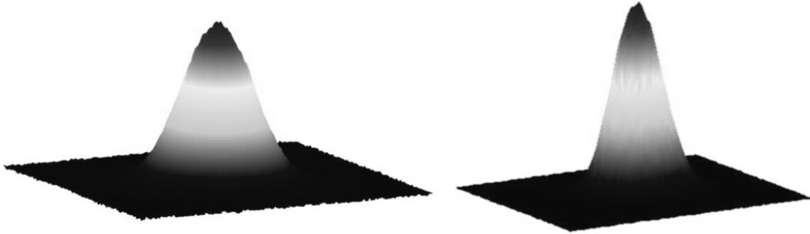
Figure 8 – Spatial profile for straight 300 μm bore guide and preservation of the SM property of the guides also depends on bending, which can couple light into higher order modes, and on the thickness of the glass wall. The most effective approach to propagating SM energy is to use a small bore waveguide, for example the 300 μm-bore by 665 μm guide for long wavelength radiation in the 10 μm range. In Fig. 8 we show the spatial profile of a straight and bent (R = 50 cm) 300 μm-bore guide. This data was taken with a CO 2 laser source launched into a 110-cm long guide. The mode remains nearly Gaussian even on bending. In Fig. 8, the profile of the bent guide appears narrower than that for the straight guide. We believe that this is due to measurement of the spatial profiles at slightly different distances from the Spiricon pyroelectric-array camera rather than any fundamental modal property. We have found that a similar experiment using the larger bore 484 μm-bore guide resulted in mode mixing and a multimode output.
