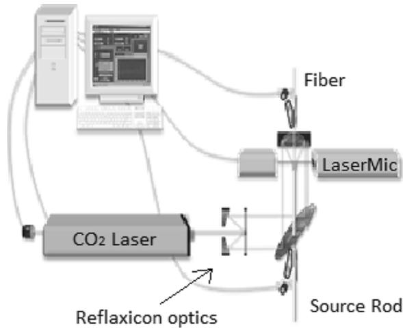
Figure 2. Schematic of LHPG.
