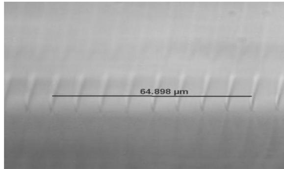
Figure 6. An optical microscope image, showing the average spacing approximately 8  $\mu\text{m}$ .
