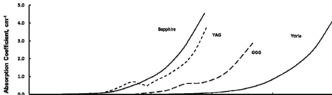
Figure 3 – IR absorption edge for bulk oxide crystals. Note the good transmission of GGG and yttria at longer wavelengths.
